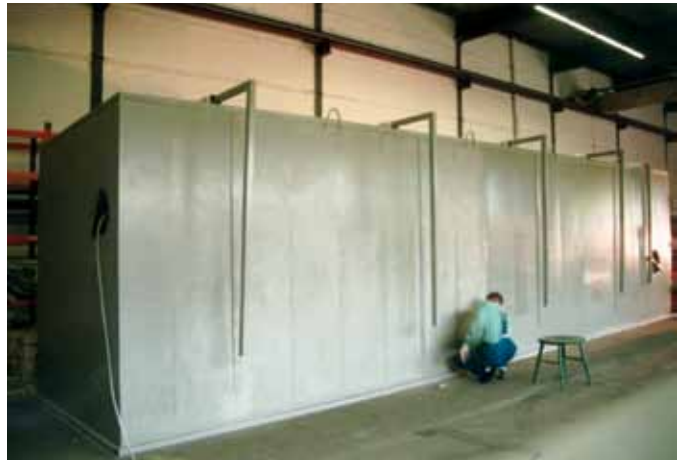
KT 36000/03/AS · Multi-chamber dryer, 36000 l volume
