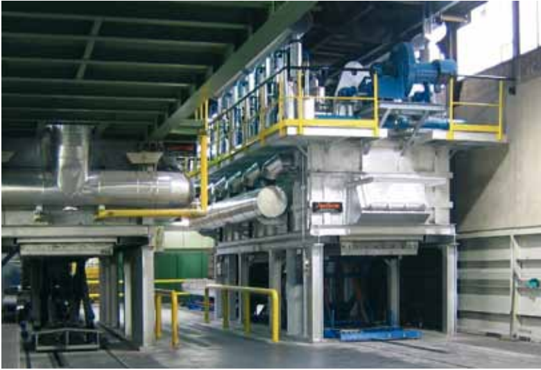
Hood furnace system · For homogenising aluminium parts
