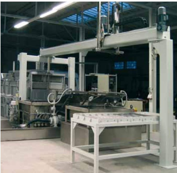
Fully-automatic system Based on a 4-chamber continuous furnace with integrated quenching and washing facility, fully-automatic batch feeding and batch transport, professional process control with extensive documentation options.
