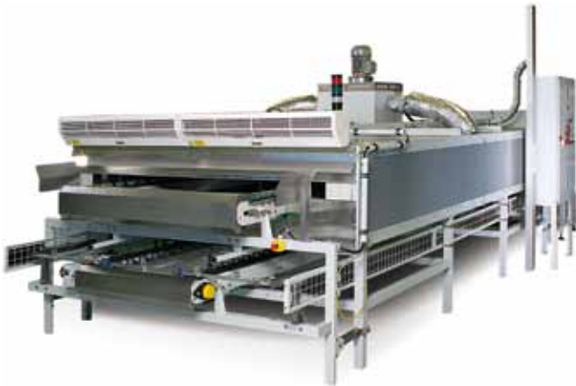
Continuous furnace DT 4700/01/AS Useable dimensions (mm): 2500 wide x 4520 deep x 420 high For hardening sealing mass on plastic housings. With extraction fans for removing vapours
