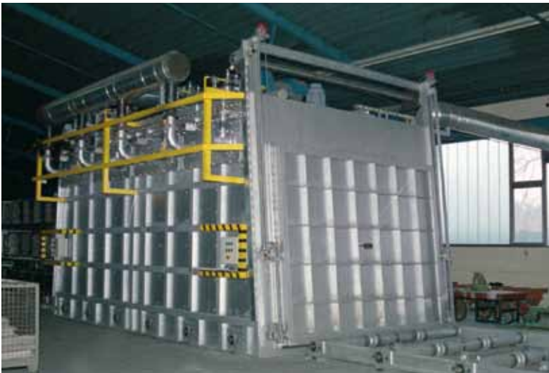
Artificial ageing furnaces · Gas fired directly
