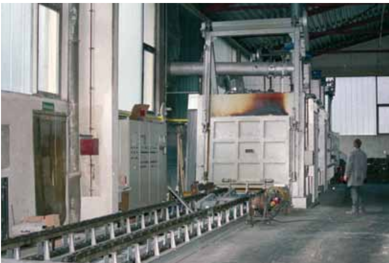
Continuous annealing furnace · With heating-up, holding and cooling chamber
