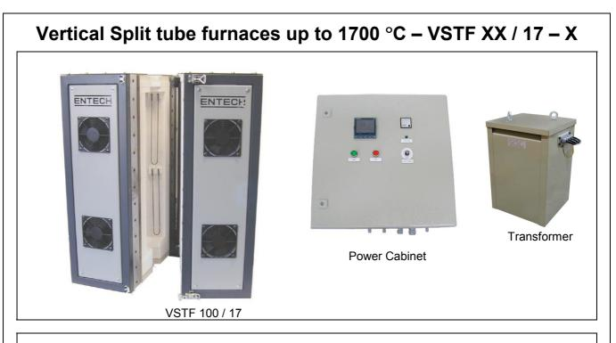
The furnace is equipped with KANTHAL SUPER 1800 Molybdenum disilicide elements. These elements offer fast heat-up rates and are able to operate up to 1700 °C without change in electric resistance due to ageing. If you need a temperature gradient or avoid it, it is possible to divide the chamber into separate hot zones. The furnaces are delivered with a bracket for wall mounting.
