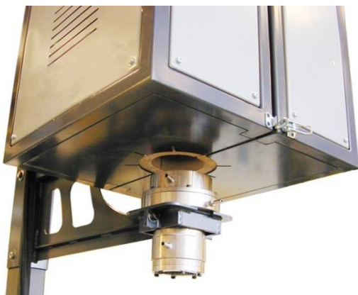
Custom made end caps to hold the ceramic tube
